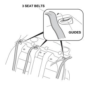
5. Open the zipper. Route the center and right seat belts through the slit in the rear seat cover.
