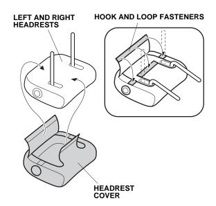
Install the center headrest cover: Fit the headrest cover over the headrest, and adjust it so that it fits smoothly over the edges. Secure the hook and loop fastener.
