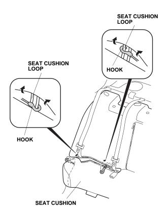
8. Pull the rear seat cover toward the left seat, and attach the two seat cover hooks to the loops on the seat cushion.
