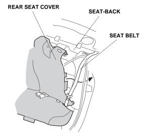
10. Tuck the four tabs into the back of the seat-back.
