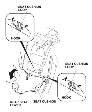
9. Route the left seat belt through the slit in the rear seat cover, then fit the entire rear seat cover over the seat-back.
